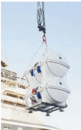
Delivered Pre-Fitted On Their Deck Cradle, The Liferafts Become Easily Portable During Installation Or Removal For Servicing By Either A Pallet Jack Or Forklift
