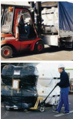
Delivered Pre-Fitted On Their Deck Cradle, The Liferafts Become Easily Portable During Installation Or Removal For Servicing By Either A Pallet Jack Or Forklift
